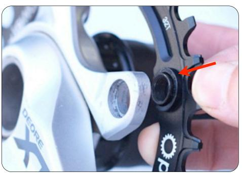
Simply add a 2mm chain ring bolt spacer on all 4 BCD mounts then mount the ring up.
