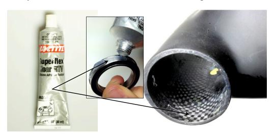
2. One side at a time, with professional press tool, carefully press M30 BB86 bearings into frame shell. The frame and bearing surfaces MUST BE PREPARED with a small amount of the required adhesive we show. See Step 1.
