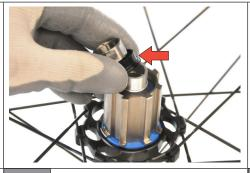
Insert the spacer and tighten the nut (Attention! The nut is left-threaded).
