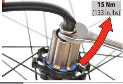
Insert the tool (UT-WHDB001 or UT-WHDB002) on the right of the axle. Using an 18 mm spanner, tighten to a torque of **15 Nm (133 in.lbs)**.
