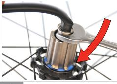
Using an 18 mm spanner, loosen the nut (Attention! The nut is left-threaded) and then remove the nut and the spacer.
