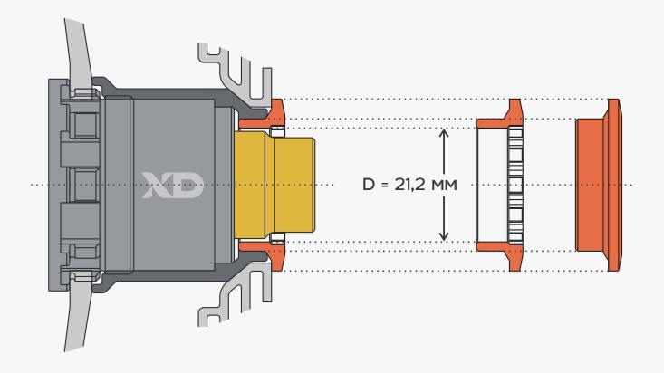
Inner diameter of Garbaruk XD-compatible cassette's outer lockring is 21.2 mm.
