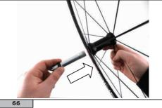
Insert the axle inside the right side of the hub body.
