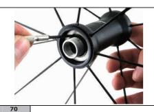
Check the cone is mates correctly into the bearing retaining ring.
