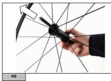
Insert the tool inside the body of the hub. Make sure you do not damage the grease shields.
