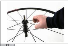
Use care not to glance off of the punch as damage can occur to the wheel.
