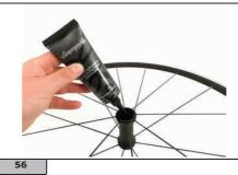
Grease the surface of the ball track of the cup using the Campagnolo grease code LB-100.
