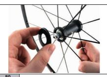
Insert the cover with the smaller internal diameter on the body of the hub on the side opposite to the adjustment ring nut.
