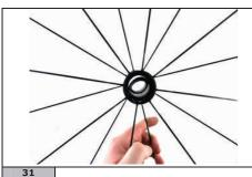
When removing the cups the grease shields may move away from their housings.
