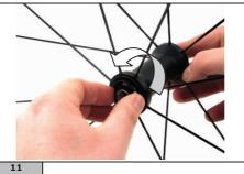
Holding the axle stationary, rotate the adjustment ring nut counter-clockwise to remove the adjustment ring nut.
