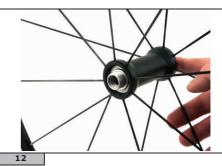
After removing the adjustment ring nut, you will see the cone and adjustment cone that we will remove in the next stage.
