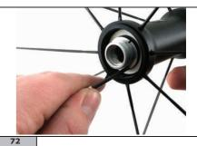
Manipulate it into position by using a small screwdriver. Push the adjustment cone in by pressing on various points of the circumference.
