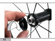
Inspect the adjustment ring nut. If it is damaged, replace it.
