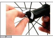
Loosen end cap (adjustment ring nut side).
