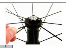
With a flat-bladed screwdriver remove the second protective cover. Make sure you do not damage the cover's locking teeth which would affect reassembling at a later stage.
