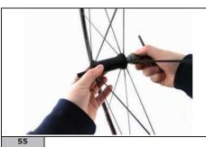
Remove the tool from the hub shell.
