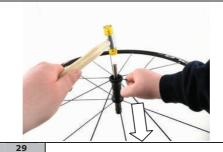
Take care to ensure that the cup stripper and punch are not propelled out of the hub when finally free of the hub shell.
