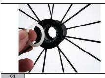
The black part of the grease seal should face the inside of the hub's body.
