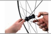
Insert the stripper inside the cup the cup that needs to be removed.
