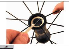
Remove the grease shield by using a small standard screwdriver. Repeat on the opposite side.
