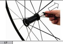
Remove the cone from the axle.
