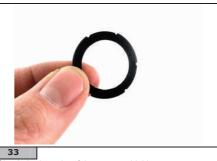
Check the integrity of the grease shield.
