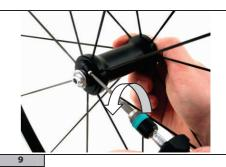
Use a screwdriver with a 2.5mm hexagon insert to loosen the screw of the adjustment ring nut.
