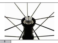
Once removed the cover, rotate the hub in the opposite direction.
