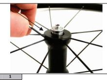
With a flat-bladed screwdriver remove the first protective cover. Make sure you do not damage the cover's locking teeth which would affect reassembling at a later stage.
