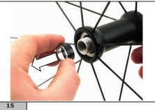
Remove the cone and the adjustment cone.
