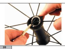
With a small screwdriver remove the bearing retaining ring making sure you do not damage it. Incorrect handling may cause the bearings to detach from the ring.
