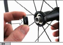
Insert the second cone onto the axle following the direction it should be inserted in. The larger diameter should face the outside of the hub's body.
