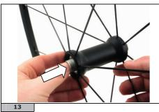
Push the axle into the hub body until it reaches the other side.
