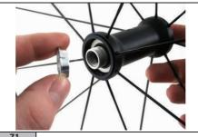
Insert the adjustment cone onto the axle mating into the cone from 69-70. The direction it should be inserted in. The larger diameter should face the outside of the hub's body.
