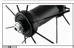
Make sure the cover engages correctly into place.
