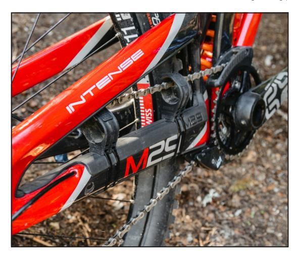
**▼ Gearing:** The STFU chain dampers are designed to work with 1 X setups only. This means if you have more than one front chain ring the system will not function as designed. We have tested using a single larger unit of the TRAIL set with 2X setups (2 front chain rings) and it works but at this stage we only offer each system as a set.
