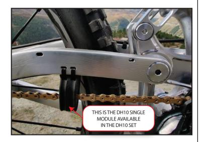
You will also need a minimum of 8mm clearance and a maximum of 60mm clearance between the chain and the chainstay when in the hardest gear (smallest cog on cassette) for the STFU to fit.
