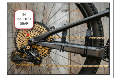
**3.** At the point marked in Step 1 - measure from the top surface of your chain stay to the bottom of your chain, directly above this point.
