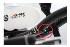
2. Adjust the computer mount to the correct height by moving the post. The top can then be rotated to the preferred angle.
