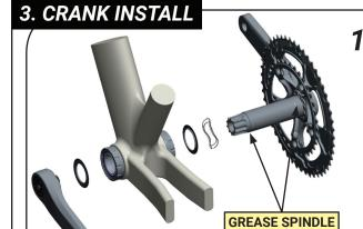
Slide the Drive Side 30mm ID Wave Washer onto the spindle.
