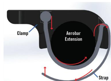
7. Tighten both mounting clamp screws to 35 in lbs (4.0 Nm).
