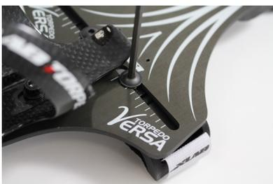
4. Place the mount on the aerobars by pressing each of the mounting clamps onto the extensions. The mounting clamp is designed to expand around the extensions and snap in place. Ensure the clamp is completely touching the extensions.
