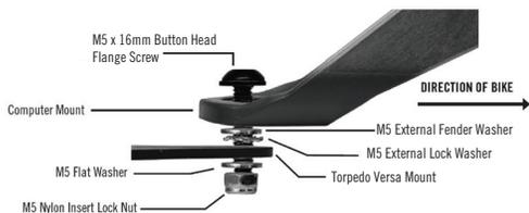
5. While holding the Lock Nut in place with the 8mm Open Ended Wrench, torque the screw to 35 in lbs (4.0 Nm).
