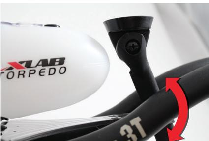
3. Tighten the side screw to lock in place and torque to 25 in lbs (2.8 Nm). The screw must be fully tightened for the computer mount to stay in place.
