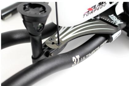
4. Adjust the position of the computer mount so the computer sits just behind the rider's wrist by sliding it forward or backwards.
