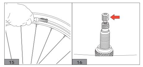
• Inflate the tyre without exceeding the maximum pressure indicated on the tyre, using a compressor or a pump, so the tyre bead is seated on the edge of the rim.
