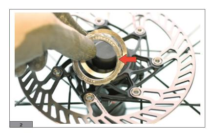
3) Screw on the locknut (Fig.3).
