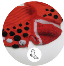
KOMPRESSIONS SOCKEN (PRO RACING SOCKS V3.0, FULL SOCKS) MATERIAL AN DER NAHT GERISSEN
