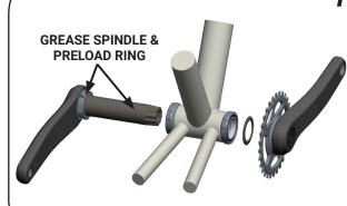
Install your specific M30 THRU BB with the correct Dustseal/ Covers for your Lyft crank. See grid on other side of instructions for Dustseal setup.
